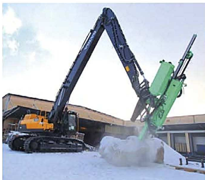
A Volvo EC480D crawler excavator adapted for drilling.
