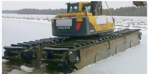
The picture on the right is the condition of the polymer track shoes working in the field for more than 5000 hours. No replacement is required.
